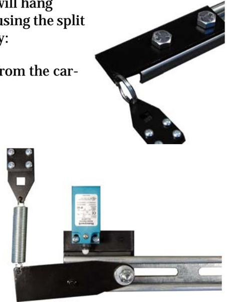
3. The assemblies to which the tape attaches, both top and bottom, allow fine alignment adjustment without having to work with the heavy, rail clamp hardware. After adjustment, torque the 3/8 bolts/nuts to 10 ft lbs.
