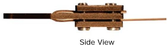
5. In the same 1, 2, 3, 4 order, make several passes, tightening each screw just a little each time. Finally, torque each screw to 14 in-lb. or 224 in-oz. (depending on the units on your torque driver). Viewed from the side, the attachment should now look as shown above — parallel plates, roughly 1/16" protruding screw threads.
