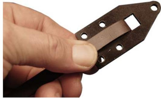
3. Place the tapped clamping piece on the back, and the through-hole piece on the top of the end piece. Hold with one hand, insert, and gently tighten one of the securing screws.
