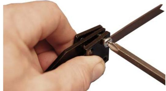
4. Next, insert and gently tighten the remaining screws in the order shown below. At this point, square up the end clamp and the tape.
