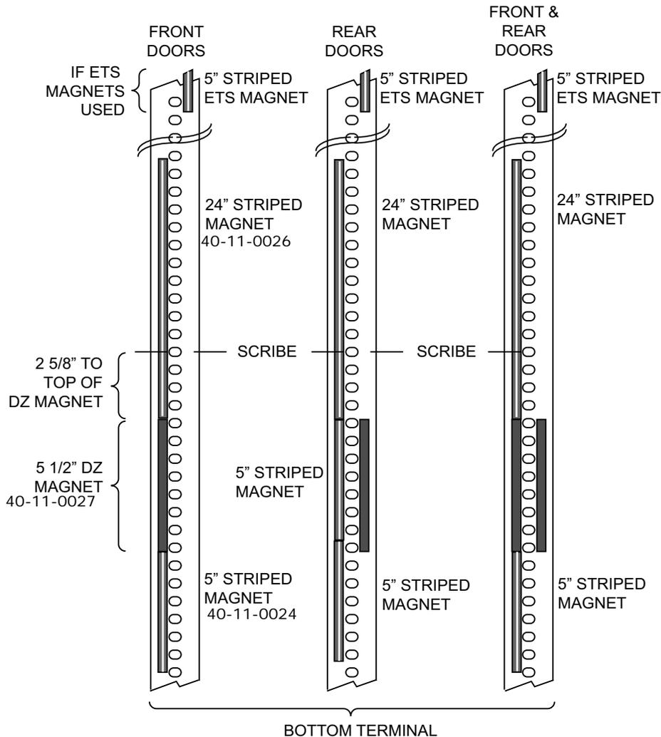
1. Place a 24-inch, striped magnet on the tape to the left of the holes, just above the bottom door zone magnet as shown above. The bottom of the 24-inch magnet must be even with the top of the door zone magnet.
