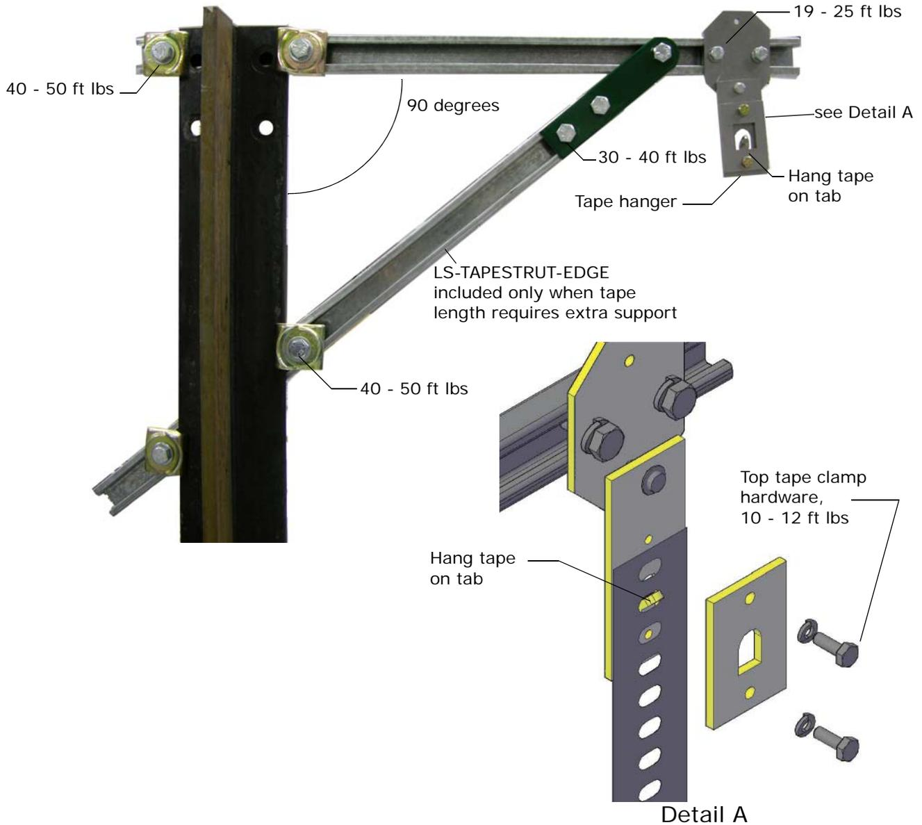
3. Adjust extended strut length as required (tape suspended as close to the guide rail as adequate clearances will allow to reduce loading on end of uni-strut). Secure rail mounting hardware (40 - 50 ft lbs.). (The tape hanger slides in the strut for fine adjustment later.)
