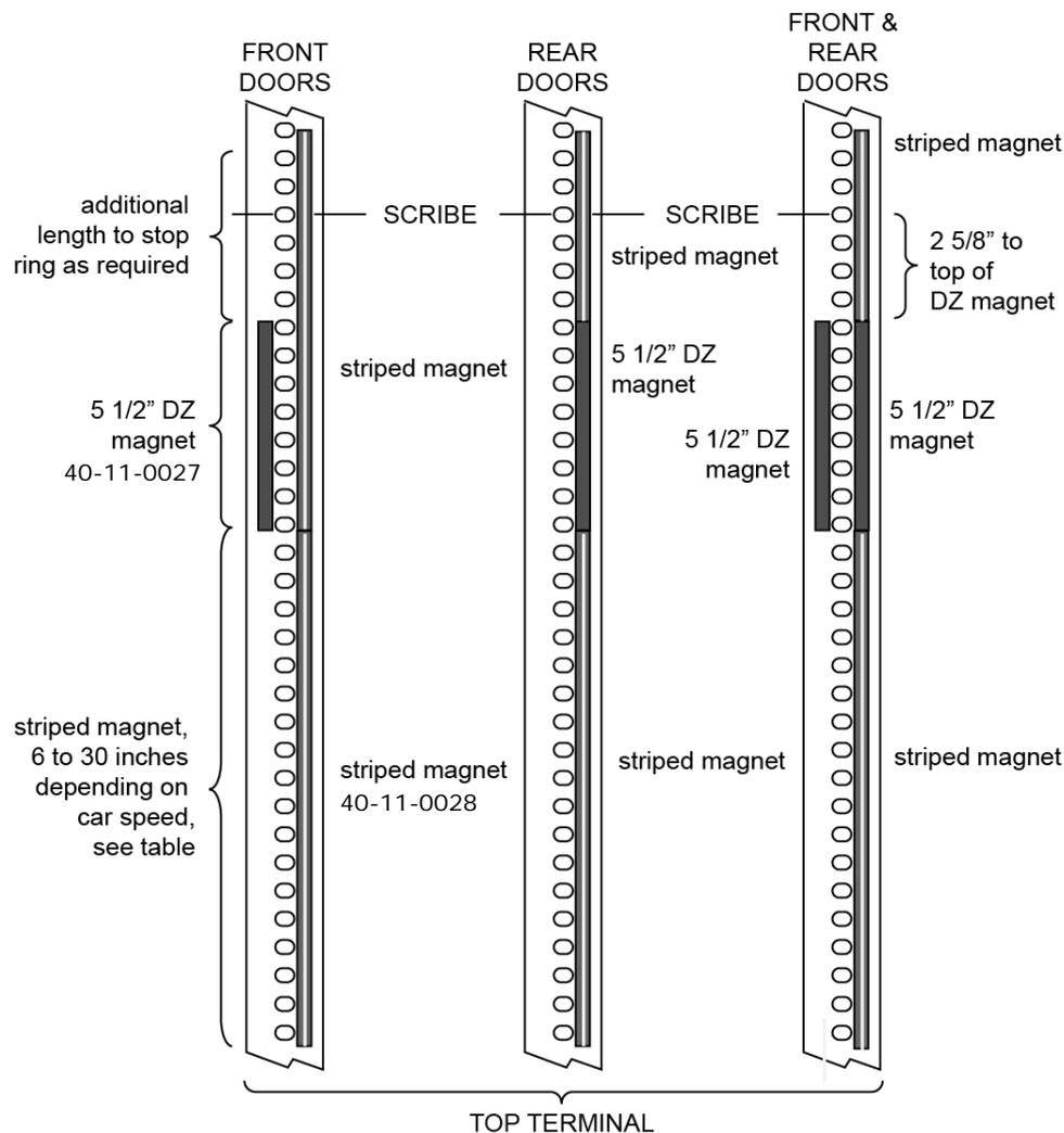
1. Refer to Table 1 on page 11 to determine the length of the magnet to be placed below the top terminal DZ magnet to the right of the tape holes ([Please refer to “Motion 2000 / Element Hydro Top Terminal Magnets” on page 10](#)).
