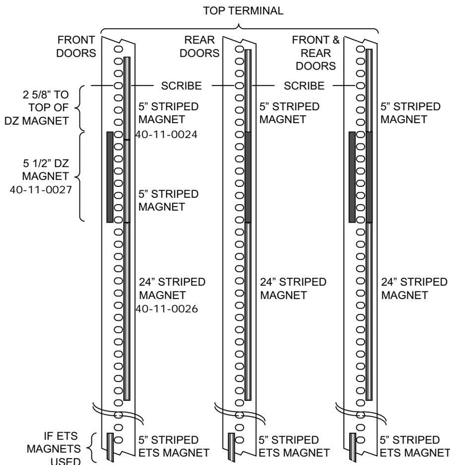
1. Place a 24-inch, striped magnet on the tape to the right of the holes, just below the top door zone magnet as shown above. The top of the 24-inch magnet must be even with the bottom of the door zone magnet.
