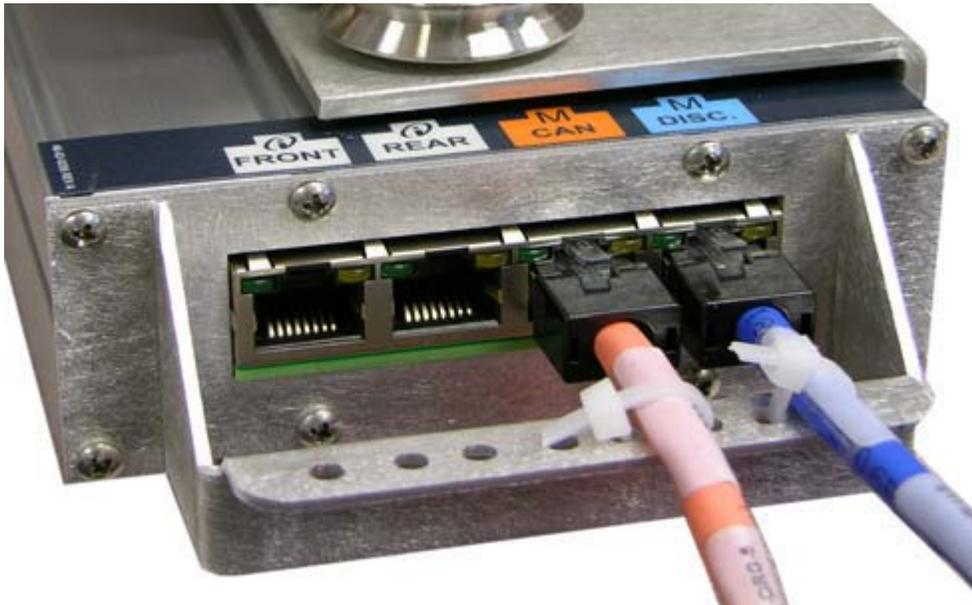
4. Cut the tie-wraps used to secure the Blue and Orange Ethernet cables. Remove the following connections from the existing LS-EDGE board.
